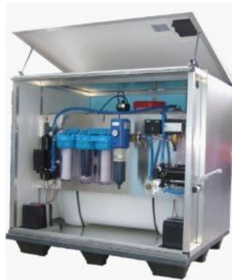
Small stationary solution with integrated drinking water storage tank and solar-cells for drinking water production for a village of about 300 inhabitants for instance (ca. 1200 l/d)
