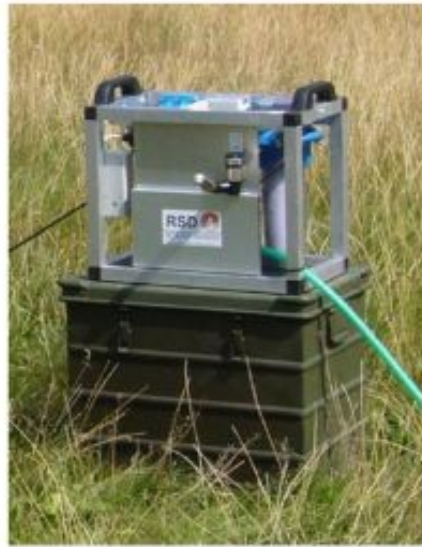
Transportable device, solar-cell powered or with car battery
